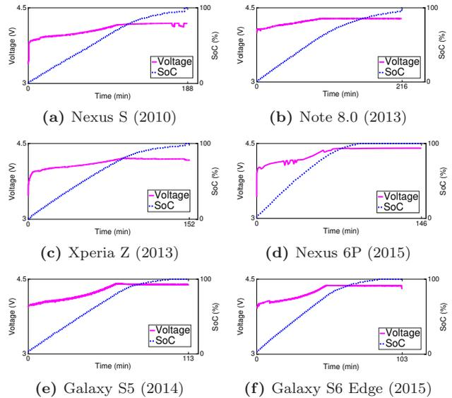
**Figure 2:** Charging mobile devices with respective chargers, showing (i) shortened charging time with the advancement of charging technologies, (ii) CCCV charging in principle, and (iii) CV-Chg takes long and is slow in charging.
