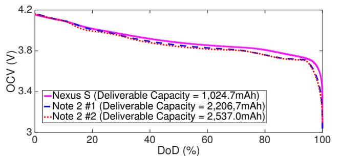
**Figure 10:** Non-linearity between battery OCV and DoD.
