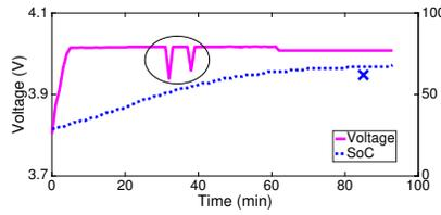
**Figure 29:** R-Aware-based charging process in Case-I on Nexus 5X.
