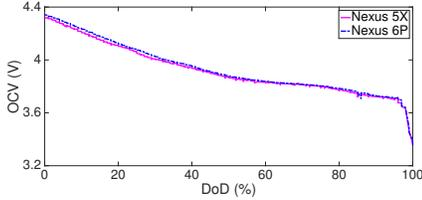
**Figure 28:** OCV-DoD curves collected from Nexus 5X and Nexus 6P.
