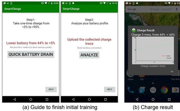
**Figure 31:** Conceptual app of iCharge. The user does one-time charging from below 5% to 95% or higher for the conceptual app to learn the battery. This charging process is displayed to the user after each charging.
