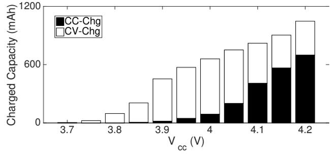
(a)  $V_{cc}$  w.r.t. charged capacity
